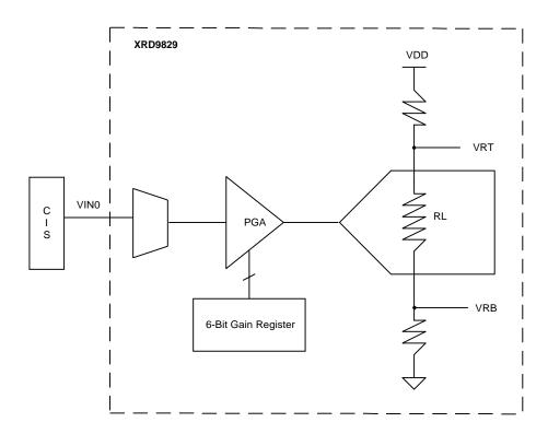
Figure 12. Simplied Block Diagram Showing Gain Adjustment by XRD9829
